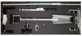
These kits contains all the torque wrenches and associated support equipment for securing the Universal Joint bolts and fixings to the correct torque. These kits are for both KIT09001 and KIT09002 technology.
